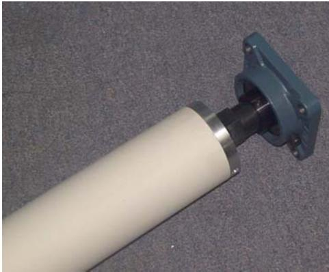
**FIXED BOWED BOWED ROLLS:** The general purpose bowed roll that fixes 90 percent of the wrinkle and stretch problems. The bow is fixed, normally at 1% of the span. Other amounts of bows are available. The roll can be rotated around its axis to help with the amount of "virtual bow". Produced in all the standard diameters, plus special, custom inch and metric dimensions.
