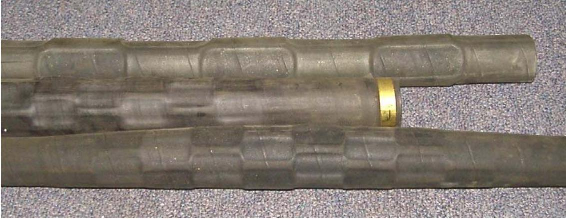
Need to replace swollen or leaking bladders? for **WEBANCOR** air shafts just supply the Shaft Serial Number. For all other makes supply us with the required I.D. O.D. and length.
