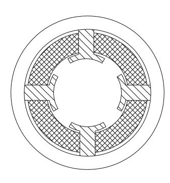
CORE I.D. AND SHAFT DIAMETER MATCHED CORRECTLY. LOAD AND AIR PRESSURE SUFFICIENT TO KEEP CORE CENTERED.
