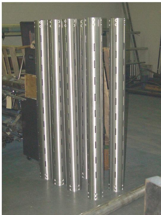
Shown here are a group of aluminum bodies ready to be assembled with the internal parts and journals.
