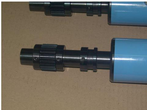
The shaft shown here is a **single bladder, rotary body type** air shaft, that is more reliable and will last longer than the multi-bladder type. While the multi bladder type shaft is advertised as being easy to repair, the down side is that it has to be repaired frequently. The bladder strips are quite expensive from the OEM.
